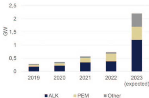
Figure 14. Current hydrogen production capacity by electrolysis in GW of existing plants worldwide 34 .
