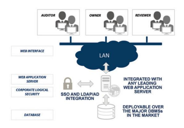
Gamma's J2EE architecture was designed strictly following standards to be deployed over the main web browsers, web servers, databases and security managers, reducing technology costs and installation time.
